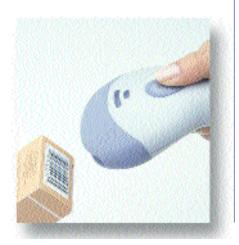
high-visibility 650-nanometer laser is automatically activated allowing the user to easily select the bar code to be scanned. Press the CodeGate button and the data is transmitted to the host system.
