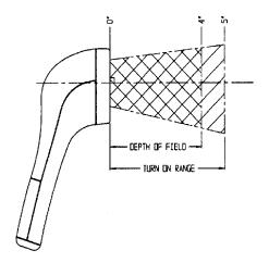
**Note:** Depth of Field based on 13mil (.013") minimum element width, Turn On Range is nominal; small variances do NOT indicate a malfunction.
