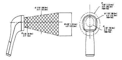
**Note:** The above scan volume shows omnidirectional volume. This volume does not reflect the entire length of all the laser lines. (Please refer to the Cross-Sectional Pattern in this section, page 20).
